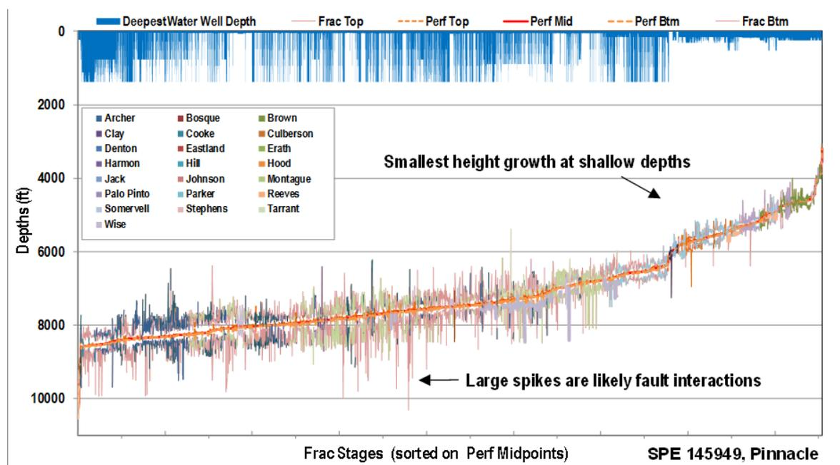
Figure 3: Data from the Barnett Shale (Texas, USA), obtained by Halliburton. Spikes represent fracture propagation depths. The tallest spikes are associated with fault linkage and propagation through pre-existing planes of mechanical weakness. The trend shows that with increasing depth, fracture magnitude increases, as a direct function of the increasing tensile strength of rocks with depth due to increasing pressure. (From Fisher, K., & Warpinski, N. 2011<sup>2</sup>)
